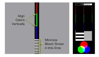
Figure 4 - Typical test patterns used for adjusting compensation
