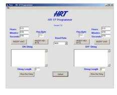
back. If you need to insert a Hexadecimal byte, you must type the Hexadecimal byte into the Hex Byte window and click Insert Hex Byte. The Hexadecimal bytes can occupy the hexadecimal range of 0x00 to 0xFF.
