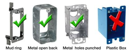
The UHBX-S-WP dissipates approximately 2.5 watts of power, so the unit will be warm to the touch, this is normal, the temperature is well within UL limits and the circuit components are designed to operate at these temperatures. Do not install the unit in a plastic electrical box, though the device will continue to operate, the elevated circuit temperature may cause the unit to fail prematurely.
