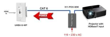
The inserter has a universal AC input and can be connected to 115~230v AC. The package and includes North American Power cord (customer must provide their own AC input cables when used with other standards).
