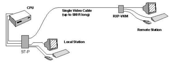
Proprietary power sensing circuit provides locally regulated power to the keyboard and mouse, and shuts them off when the PC is turned off. All keyboard and mouse data are double-buffered in order to allow extended cable lengths to 500 feet.
