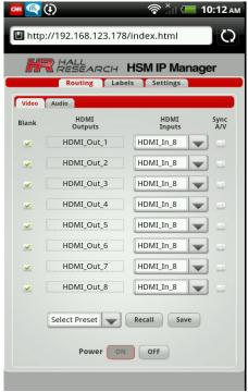
Figure 11 - Video routing sub tab
