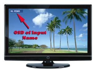
Figure 6 - On Screen Display of user defined input names after switching (position and duration is configurable)
