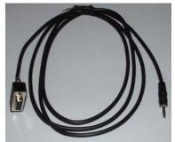
Connect the HR-1P to the PC's comm. port you selected earlier via the supplied programming cable. The supplied programming cable is a 6' cable that has a female DB-9 connector that connects to the PC and the other end is a male mini-stereo connector that plugs into the HR-1P.
