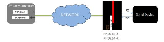
To perform a full Duplex SoIP with FHD, the 3rd party controller requires the following Client and server architecture.
