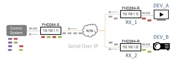
MCD at the Receiver can reduces the load on control system caused due to parsing by aggregating the data from the serial device in a buffer and send it to the sender as a complete response.
