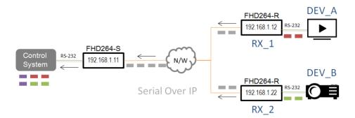
Enabling **Packet Mode** at TX will append a <u>header</u> to the received payload from a receiver, which allows the Control System to parse (Differentiate) the responses from the SOIP devices attached to the receivers.
