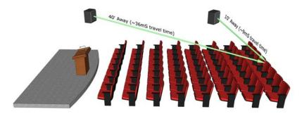
The AD-340 Audio Delay Processor is designed to provide a flexible way to adjust for these types of delay by adding a digital delay function based on 5 different delay types.
