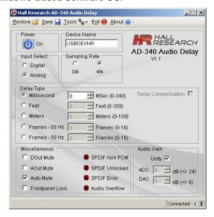
The AD-340 Programmer is a software-based solution capable of configuring any setting on one or more AD-340 devices connected to the Windows PC via a valid USB connection.
