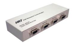
The Model 400-DX provides amplification of video signal with very high bandwidths (exceeding 250 MHz) to ensure operation at up to 1600x1200 pixel resolutions. As noted earlier, Outputs #1 & 2 have special gain and frequency compensation for connection to long cables.
