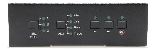
The SEL INPUT button and A/B/C LED indicators select which line input on the rear panel is mixed into the MIC INPUT, RCA, 3.5mm or SPDIF inputs respectively.
